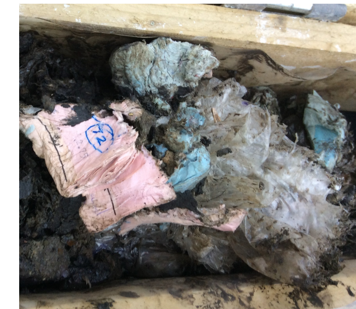
Figure 4b: Example of more modern waste containing paper and plastic packaging material.
