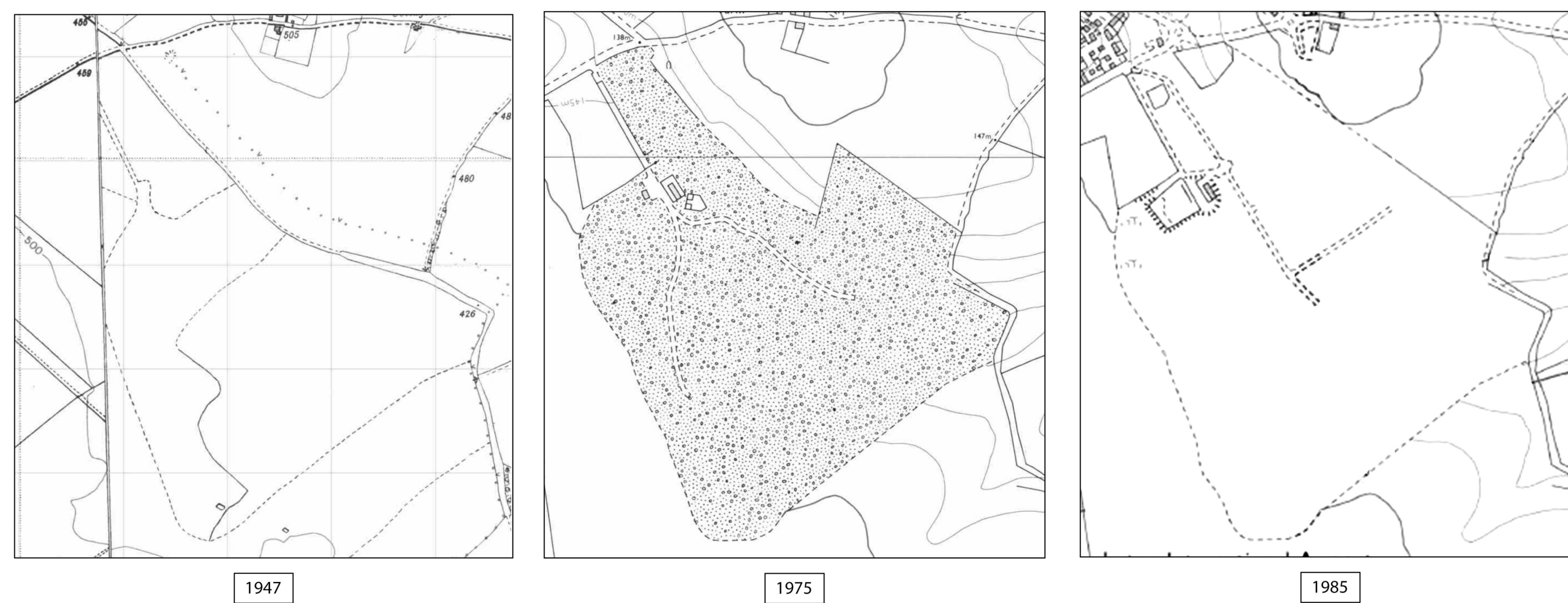
Figure 1 : Use of historic mapping to create a digital surface of the filling history of the landfill
